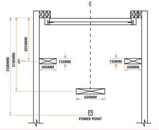
NOTE: THE DETAILS SHOWN ARE FOR 2.3M MAXIMUM HEIGHT SECTIONAL DOOR WITH STANDARD 350MM HEADROOM.
