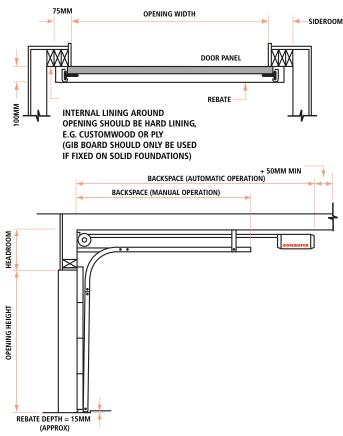
NOTE: 1. FOR AUTO OPERATION POWER POINT AND BELL WIRE TO BE FITTED 3.3M BACK FROM CENTRE OF OPENING. BELL WIRE TO BE RUN TO NEAR ACCESS DOOR.
