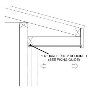
Longer boards that require two or more fixing points (in addition to the fascia slot) should have one 'hard fixing' closest to the fascia board and then remaining fixings to be 'standard fixing'.
