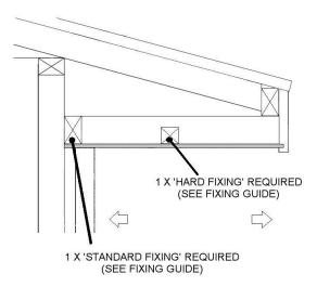
Board lengths exceeding 1500mm are to be 'mid fixed' approximately half way along the board.
