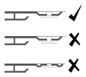
DO NOT FIX THROUGH A PARTIAL SLOT. If a slot is cut through at the end of a board, fix in the nearest full slot. See below.
