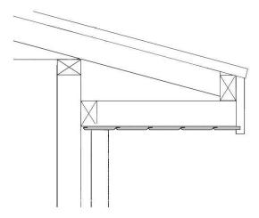
Starting and finishing of cut boards can be achieved by using the end cap accessory or the installation of an alternatively supplied moulding.
