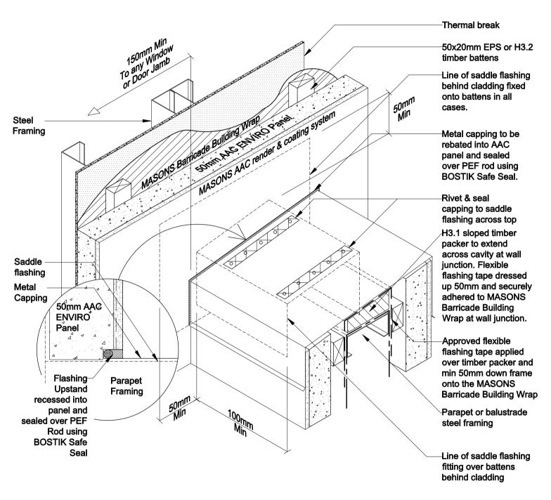
PARAPET / HANDRAIL TO WALL JUNCTION With Metal Capping - 3D View
