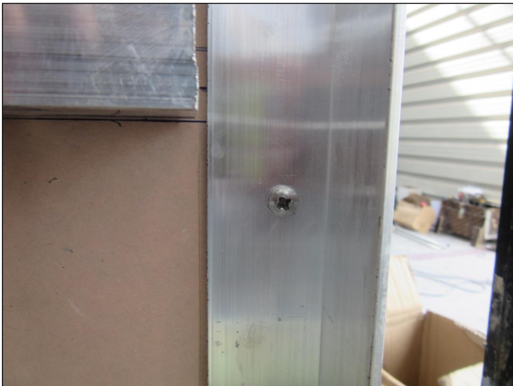
Picture 2: Aluminium L-angle along the vertical edge of the specimen.
