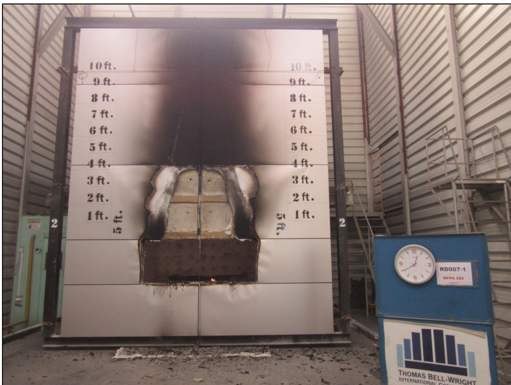
Picture 16: The specimen at the end of the observation period and end of the NFPA 285 test.
