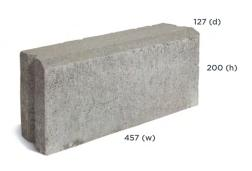
Firth Road Kerbs are designed to create the kerb on road network pavements. They can also be used to form the perimeter to car-parks and access ways. Firth Road Kerbs are laid in a concrete haunch with the V joint between units filled with mortar so they lock together.
