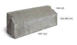
Firth Mountable Kerbs are used to form road edging and are ideal to form the edges of traffic islands and crossings. Mountable Kerbs have a sloping face rather than an abrupt angle and this enables vehicles to drive over them easily. Laid in the same way as Firth Road Kerbs.
