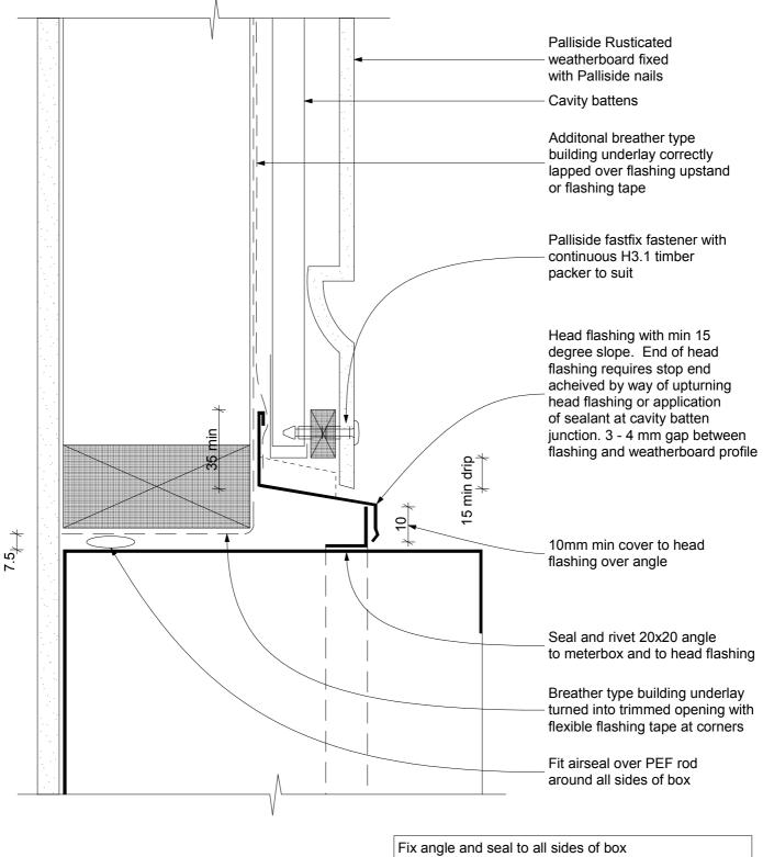
At sides and base cladding shall overlap by 10mm This detail is also suitable for other similar penetrations
