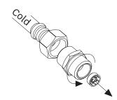
All pipework must be thoroughly flushed prior to the installation of the mixer. In-line filters must be fitted on both hot and cold supplies to prevent foreign particles damaging the ceramic cartridge.
