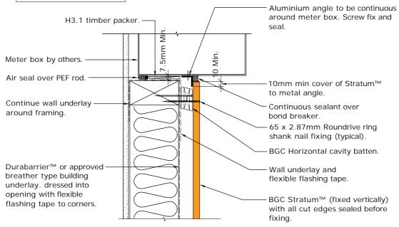
Note. Where Durabarrier™ is used flashing tape must be applied to the entire opening
