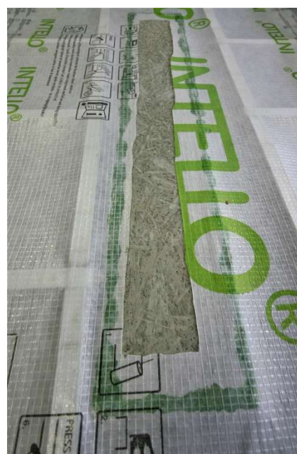
Fig. 1: Membrane to concrete connection using ORCON F in the test apparatus (left). Membrane to concrete connection in detail (right).
