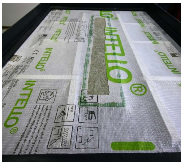
Fig. 1: Membrane to concrete connection using ORCON F in the test apparatus (left). Membrane to concrete connection in detail (right).
