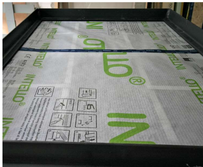
Fig. 1: Connection membrane to membrane with TESCON VANA in the test apparatus.
