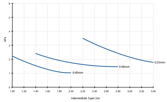
Note: The intermediate spans shown in the graphs above are based on G550 Steel as the base metal. To calculate end spans please multiply the intermediate span calculated by 0.66. Spans are based on restricted access. For alternative metals please contact your local Metalcraft branch.
