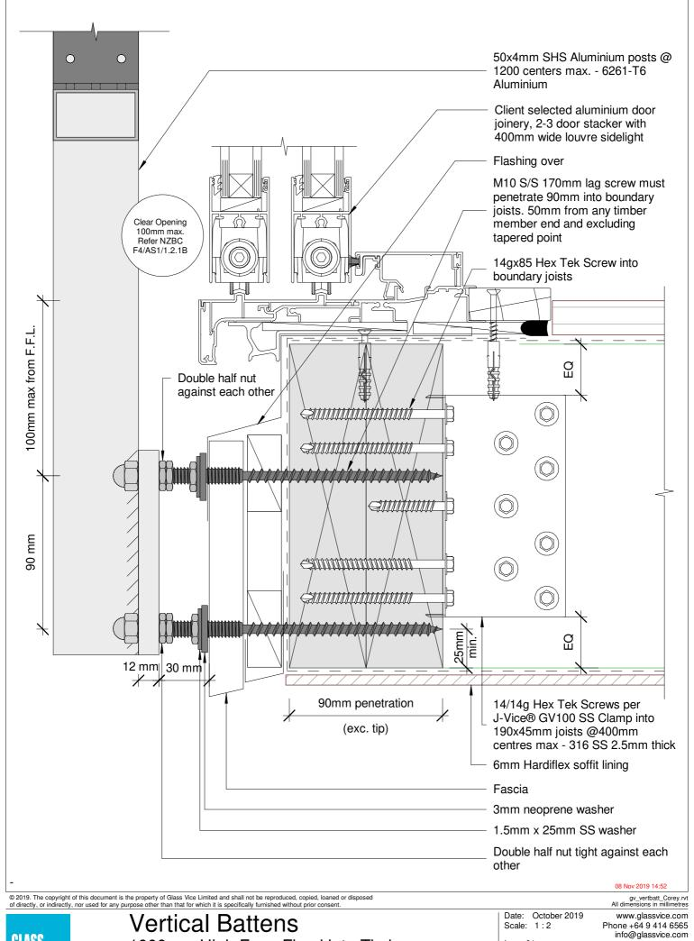
1000mm High Face Fixed into Timber Detail - Face Fix 190 Double Joist with Door
