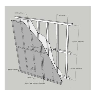
Diagram: Batten and Fibre Cement board set-out
