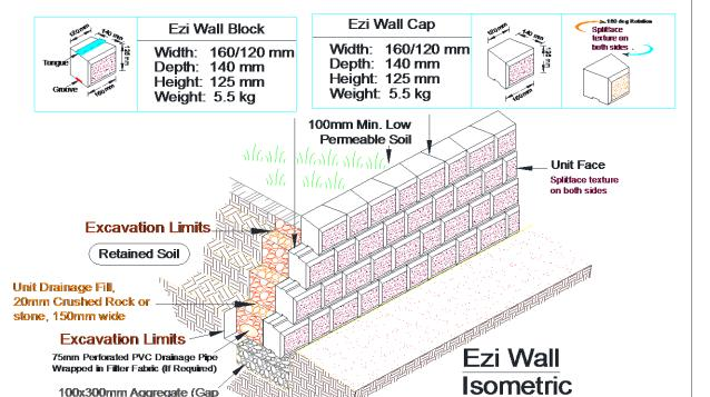
100x300mm Aggregate (Gap 20) Compacted Leveling Pad
