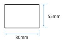
THERMOCLICK CHANNEL JOINER PLATE - Connected with riverts or small screws
