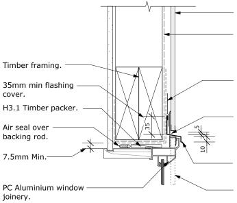
BGC Duragroove™ with all cut sheet edges sealed before fixing.
