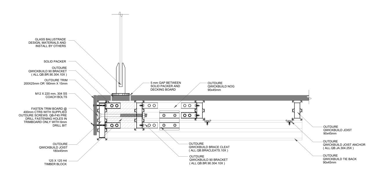
QB-G3. BALUSTRADE PARALLEL TO JOIST DIRECTION FOR 90mm JOIST ( SECTION VIEW 2)
