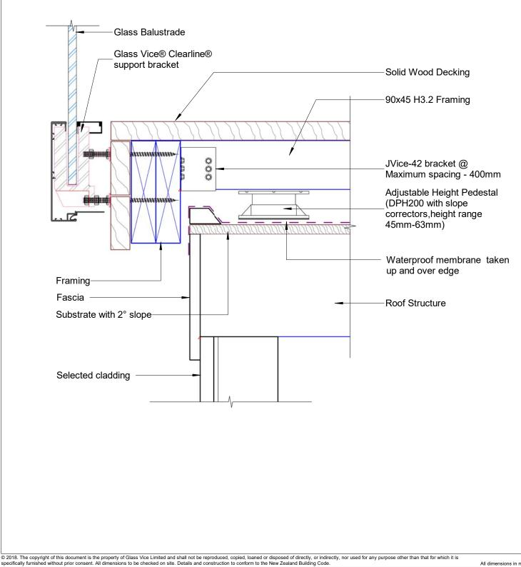
GLASS Vice Glass Vice® Deck Overlay 100mm to 190mm Raked Joists With 250mm Maximum Overhang Side Edge Detail Clearline Date: 9/7/18 Scale: 1:5 Version 4
