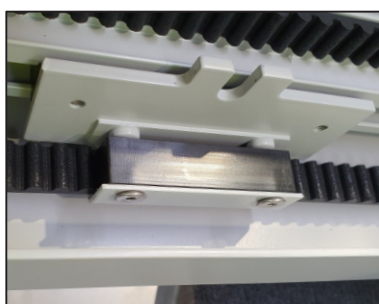
Belt pulled out of the way, to show Clamp
