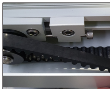
Belt pulled out of the way, to show Idler Pulley Assembly
