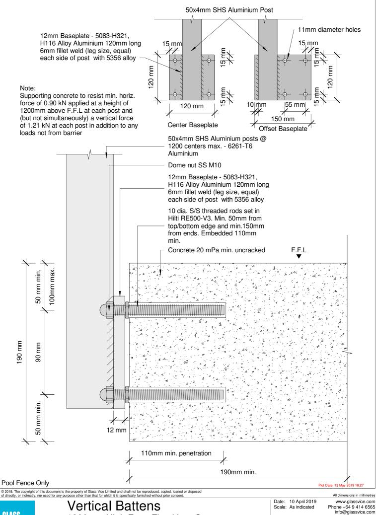
1300mm High Face Fixed into Concrete Detail - Face Fix Concrete 1.3M Pool Fence Only
