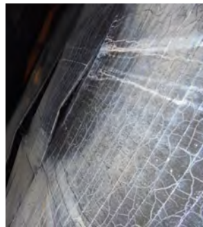
Fire penetration into panel core, material charred but still in place, no void.
