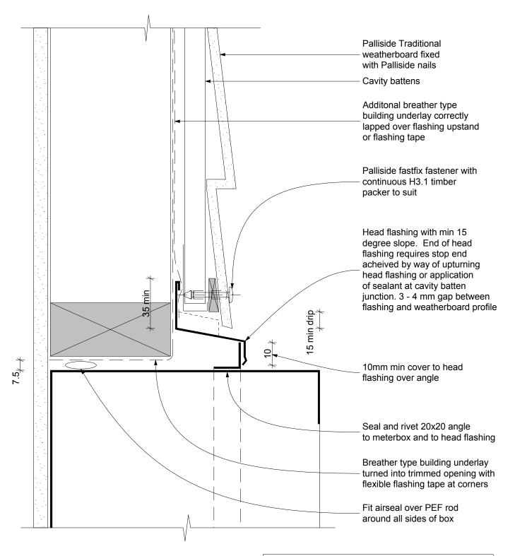
Fix angle and seal to all sides of box At sides and base cladding shall overlap by 10mm This detail is also suitable for other similar penetrations
