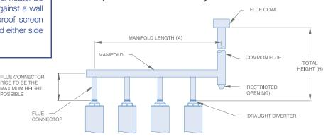
Multiple Manifold Flue System
