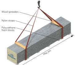
The recommended lifting method for bundles no more than or equal to 6m can be handled with a crane by using nylon straps and wood spreaders as shown.
