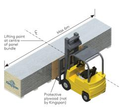
The recommended loading / unloading method for bundles less than or equal to 6m is to use a single forklift with widely spaced forks placed under the centre of the bundle as shown.
