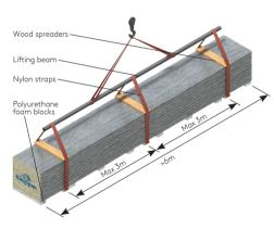
The recommended lifting method for bundles more than 6m, by crane, is by using three points of support. To prevent damage from nylon straps, use wood spreaders at top and bottom at lifting locations as shown.
