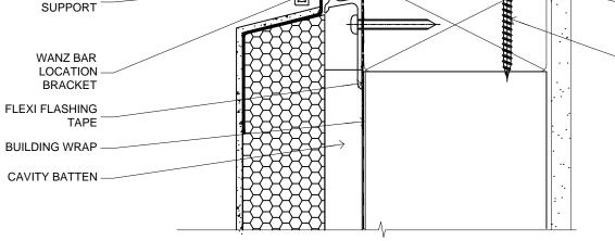
FLAT PACKERS FIXINGS: PAIRS OF 75x3.15mm NAILS OR 1 X 8g 65MM SS SCREWS AT 150 FROM CORNERS AND 450 CENTRES
