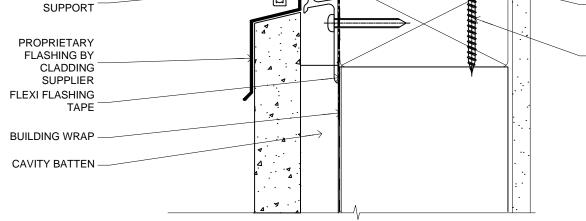
FLAT PACKERS FIXINGS: PAIRS OF 75x3.15mm NAILS OR 1 X 8g 65MM SS SCREWS AT 150 FROM CORNERS AND 450 CENTRES
