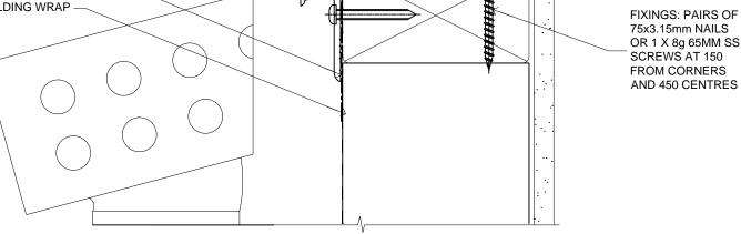
FIXINGS: PAIRS OF 75x3.15mm NAILS OR 1 X 8g 65MM SS SCREWS AT 150
