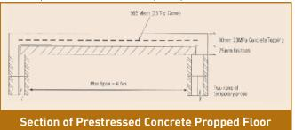
panels/beams with a concrete topping poured on site. The units are available in lengths to suit the project design and must be placed as per the construction drawings prepared by the supplier. The units are uniquely identified for this purpose.
