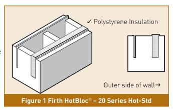
the simplest means of compliance as the insulation is built in. It affords the structural strength of standard masonry (see 1.5 Engineering below) as well as providing options to meet the R-values stipulated in the Building Code for solid construction, refer section 1.6.
