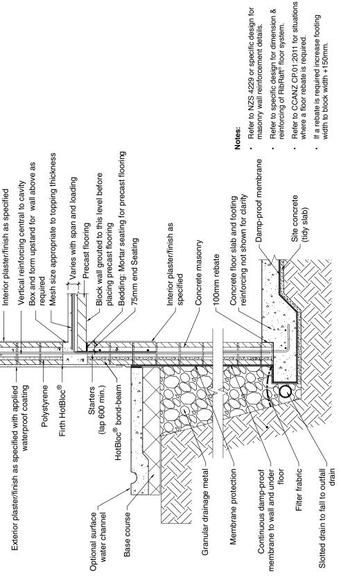
Note: refer to NZS 4229 or specific design for masonry reinforcing
