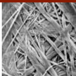
Figure B – DuPont™ Tyvek® fibers (magnified 75x) form a strong web that maintains excellent breathability and water holdout.
