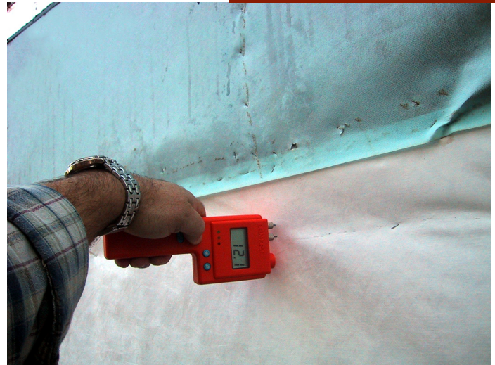
High vapor permeable housewrap with low moisture reading on OSB under the DuPont™ Tyvek® HomeWrap®
