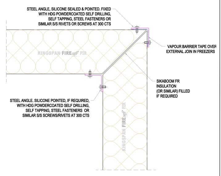
(T & Y) TYPICAL MITRED EXTERNAL COLDSTORE CORNER JOINT DETAIL
