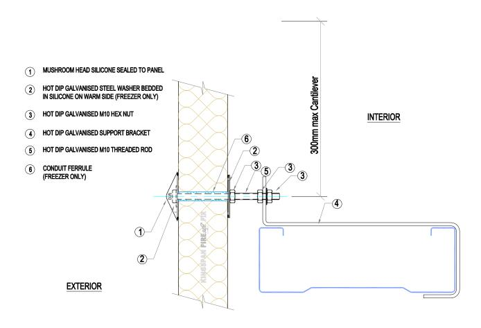
(H, I & X) TYPICAL INTERMEDIATE WALL PANEL SUPPORT FIXING DETAIL FOR EXTERNAL COOLSTORE WALLS (VAPOUR BARRIER SEALED & POINTED WITH GUN GRADE SILICONE TO WARM SIDE OF FREEZER WALLS)
