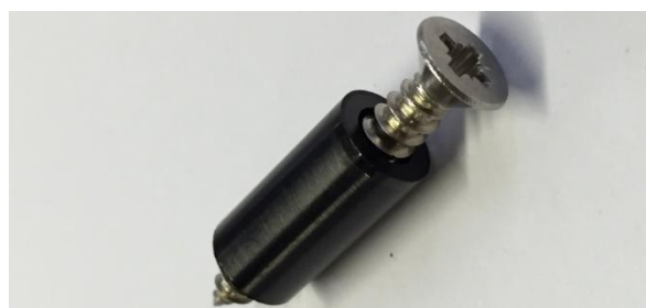
Insulator for mounting screw to prevent damage to adjacent supply wiring.
