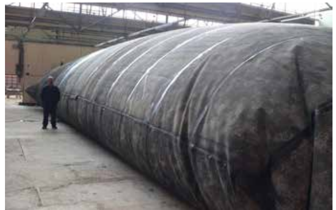
A pillow tank inflated for testing purposes in the Christchurch manufacturing plant.
